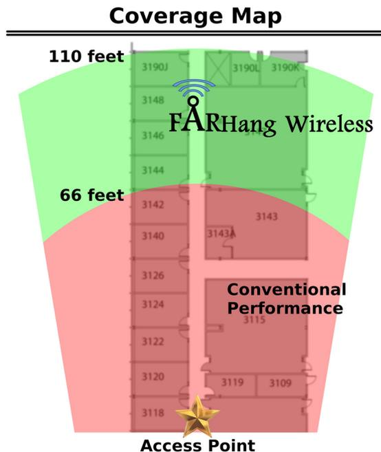
Figure 4: Real-world results showing performance in an office environment.
